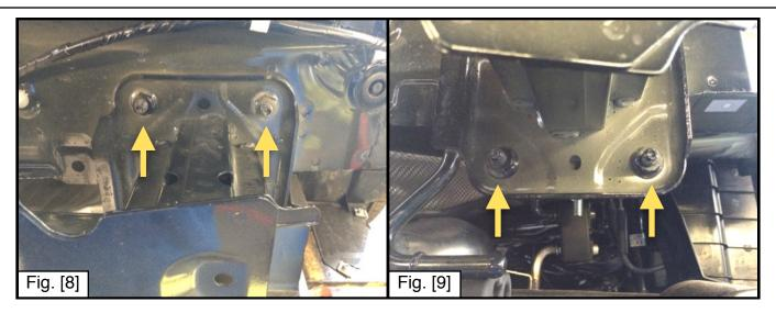
**Step 5.** Hang the EcoHitch onto the impact bar stud bolts and replace the impact bar over the EcoHitch. Secure with the factory nuts and hand tighten. Once the EcoHitch is centered, torque the hardware to 40ft-lbs.
